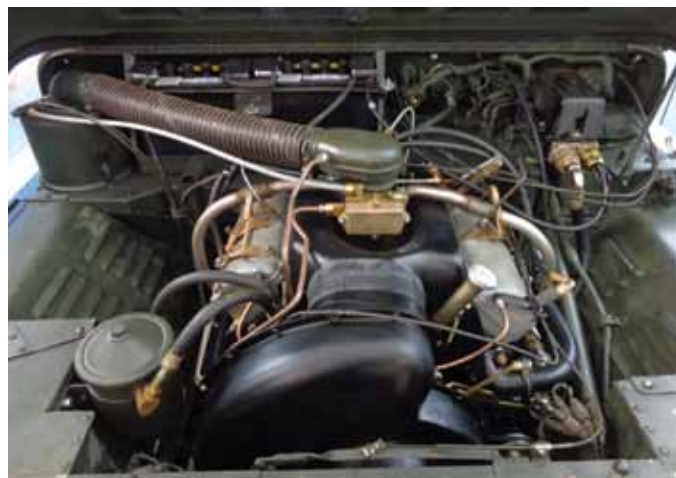
The Mite has a lot of hard oil lines to route oil, all the OEM vacuum lines on the Mite are plastic and a breeze to install.
