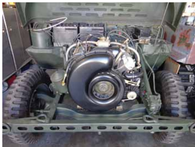
Getting the power pack in a mite is a tight fit, one trick is the remove the brake drums on the front differential before installing....a little extra clearance goes a long way.
