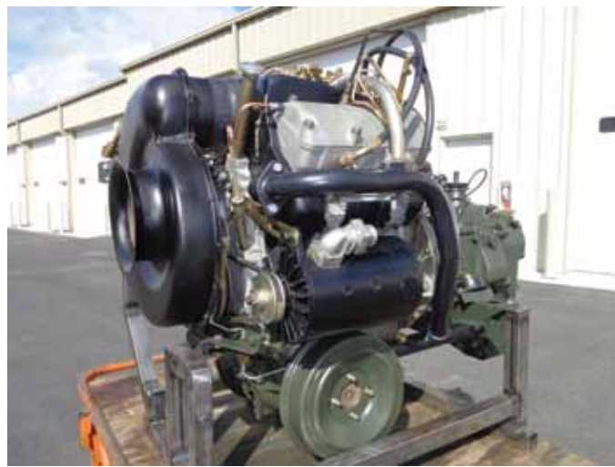
Complete Power Pack ready to go back into the mite....) If possible, it is nice to test run it for leaks before it goes in.
